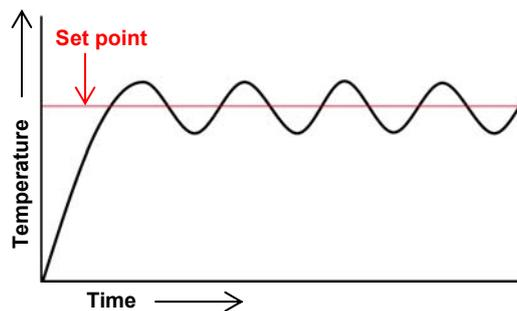
The duration of the calling period is governed by the sensitivity of the sensing element (the bigger the better) the speed of the reaction of the sensing element, the siting of the thermostat and the design of the rest of the heating system.
